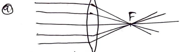
When parallel beam of light incident on a convex lens parallel to principal axis, they converge to a point on the principal axis  $\Rightarrow$  principal focus.
