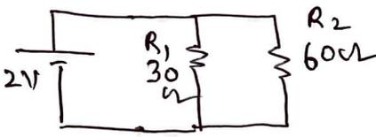
$$R = \frac{R_1 R_2}{R_1 + R_2} = \frac{30 \times 60}{30 + 60} = 20 \Omega$$
